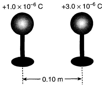
The spheres are touched together and then returned to their original positions. As a result, the magnitude of the electrostatic force between the spheres changes from 2.7 N to
