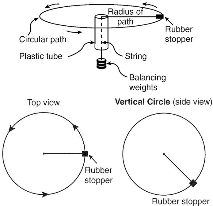
4. The rubber stopper is now whirled in a vertical circle at the same speed. On the diagram, draw and label vectors to indicate the direction of the weight ( $F_g$ ) and the direction of the centripetal force ( $F_c$ ) at the position shown.
